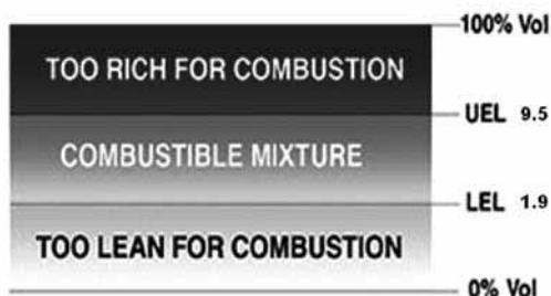
Fig-2 - Flammability limits of LPG
